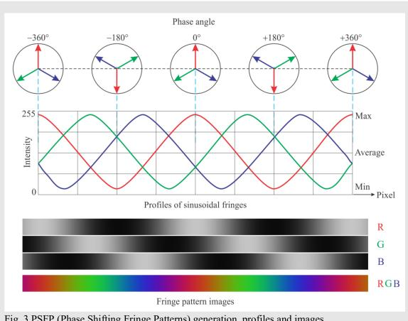
Fig. 3 PSFP (Phase Shifting Fringe Patterns) generation, profiles and images
