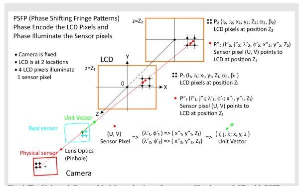
Fig. 1 The Universal Camera Model, mechanism of camera calibration, an LCD with PSFP on a linear stage. The location of the camera is fixed. The locations of the LCD can be at 2 or more.
