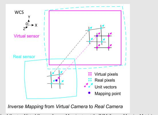
Fig. 4 Create a Virtual Camera. Inverse Mapping to get the IMM (Inverse Mapping Matrix)
